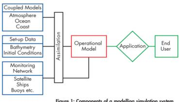
Figure 1: Components of a modelling simulation system
